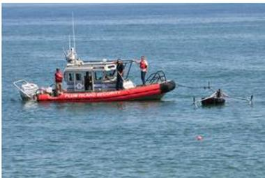
Stevens Research Engineers work in conjunction with Plum Island Animal Disease Center (PIADC) personnel to deploy passive acoustic detection devices adjacent to Plum Island in a recent experiment.
